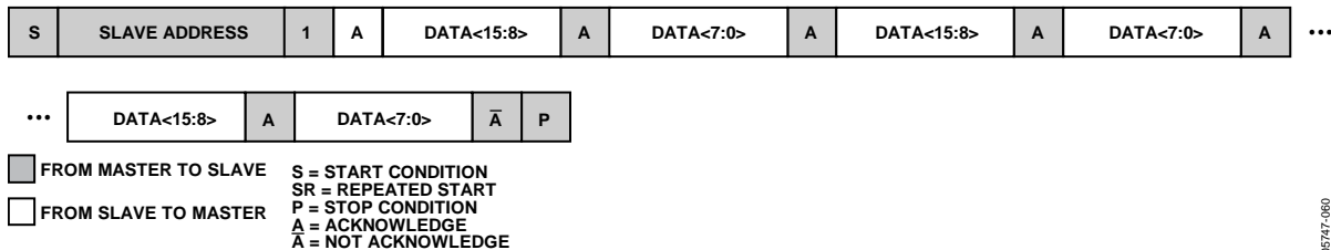
Figure 14. Reading Three Lots of Two Bytes of Data from the Conversion Result Register
